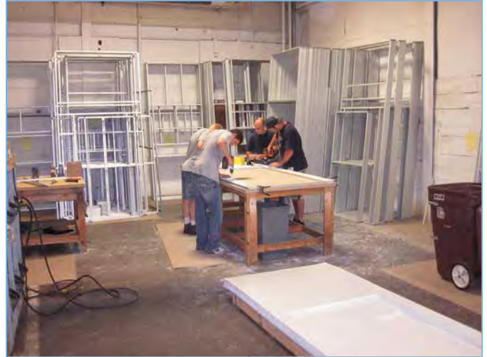
Fabrication of cage panels in the shop
